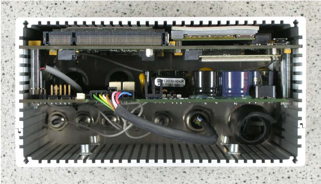
NB3711-L2Wac-G-AE, rear cover removed: PSE_Board 5x_M12_front in the middle, MC board on top
